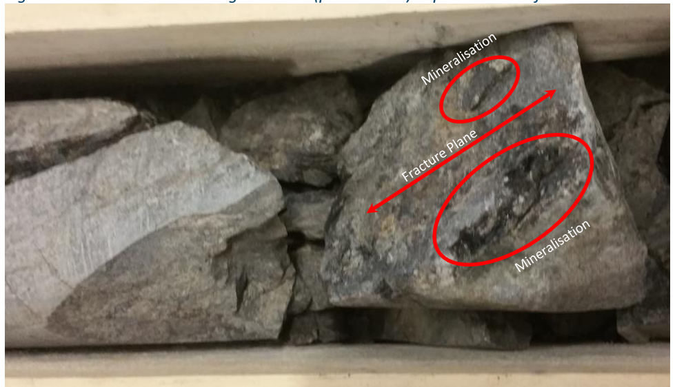
Figure 5: Retortillo ore showing uraninite (pitchblende) exposed in rock fracture
